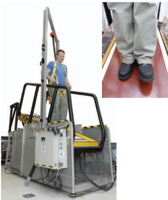
Figure 4 The UKSRG ramp CoF test
